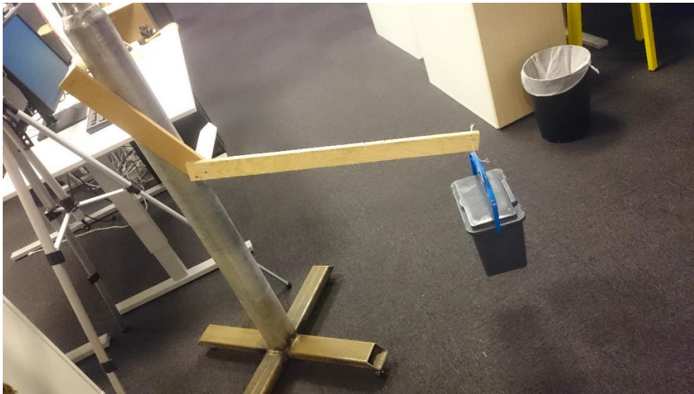
Figure 7-3 Rudimentary prototype for a leverage type climber.
