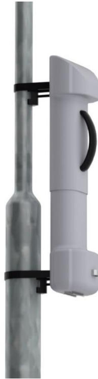
Figure 14-3 Possible future design for a pole climber.
