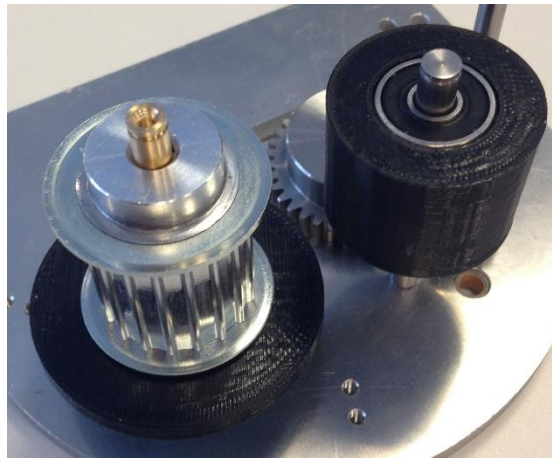
Figure 12-12 Timing belt pulley for collecting the cog belt.
