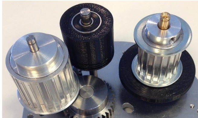
Figure 12-13 The timing belt pulley for the cog belt drive seen on the left.
